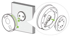
**Step 3:** Attach the bracket on the wall using the wall mounting screws.
