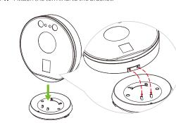
**Step 2:** Tighten it with a desktop bracket screw.
