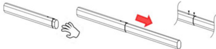
Figure 1 Connect the main boom arm with the Secondary arm together by 2 screws
