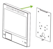
5 Secure the Kiosk by assembling the device and the rear panel with the bottom screw.
