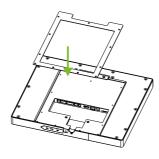
2 Secure the plate with the screws (11 pcs) to the back of the unit.
