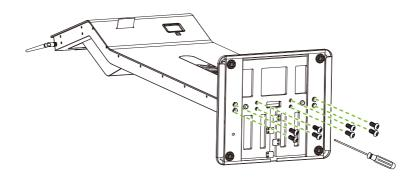
3 Place the device in the right position and remove the four screws that secure it to the base, remove the metal cover.
