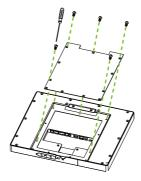
3 Place the rear panel at an appropriate height from the ground. Drill the holes on the wall and fix it.
