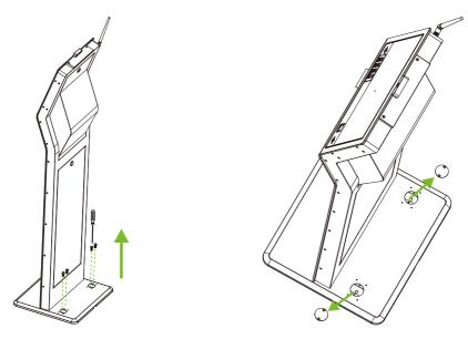
4 Drill holes with an electric drill, implant two screws into the ground to fix the device, then cover back the metal cover, and finally tighten the four screws.
