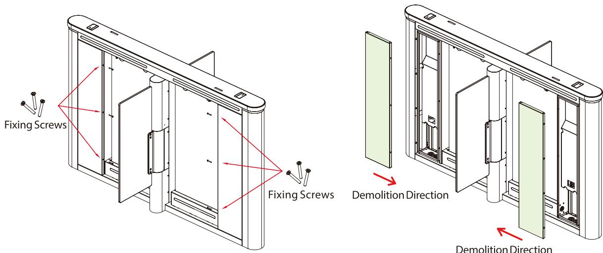
2. Using a Phillips screwdriver, remove the three fixing screws at the locations shown below, then take off the cover plate.
