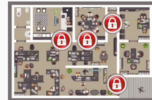
Administrators can remotely open/close and/or lock down all, selective doors or group of door on the system. When the “Active Lockdown” command is activated, all doors will be locked at the same time
