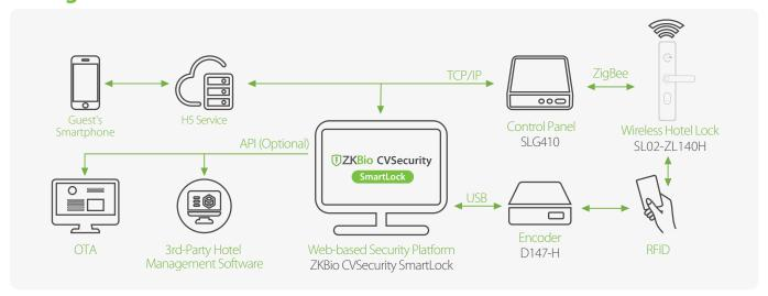
Note: It illustrates a complete hotel lock management system for ZKBio CVSecurity SmartLock and provides commonly used API interfaces.
