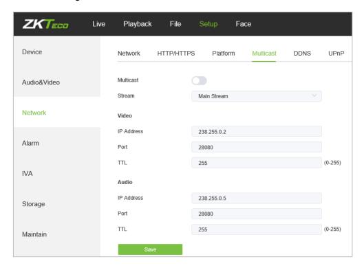
Multicast configuration is disabled by default. By clicking on "Enable Multicast", users may set the IP address, port and TTL of main stream video/audio, sub stream video/audio.
