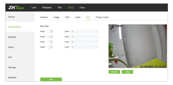
• ROI Settings: On the preview window, hold the left mouse button and drag to set the ROI area. There are a total of four ROI areas available. Click on to set the corresponding ROI region coding level; the higher level the coding, the stronger the ROI region encoding.
