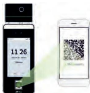
**Note:** Place your phone within **15 to 50cm** of the device (distance depends on the size of the phone screen), do not block the device QR code scanner and QR code in the phone screen.
