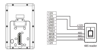
**Note:** 485A and 485B can be connected to the Barrier gate or the 485 Reader, separately, but cannot be connected to the gate and reader at the same time.
