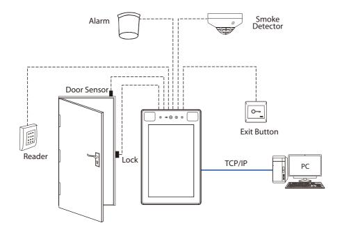
5 Door Sensor, Exit Button & Alarm Connection
