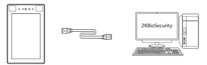
Default IP address: 192.168.1.201 Subnet mask: 255.255.255.0 IP address: 192.168.1.130 Subnet mask: 255.255.255.0
