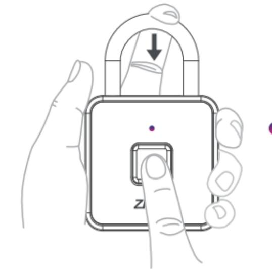
Under the locked state, push the U-type shackle to its lowest position (just a little bit down). Touch the fingerprint sensor, **blue and red LED** will light, which means the lock enters deletion mode.
