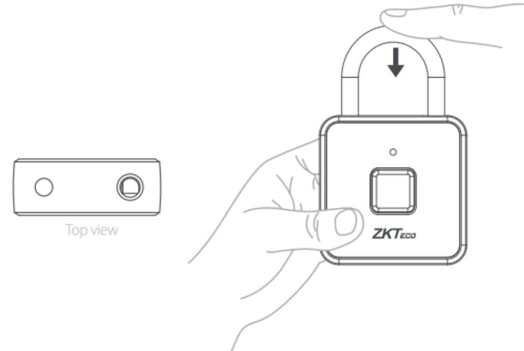
Press down the U-type shackle to the hole, and it will be locked up.
