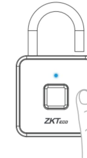
Then move off the finger and **blue LED** will blink, which means the lock enters registration mode.
