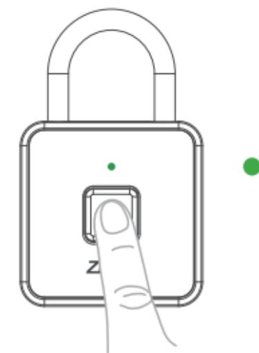
Press with one finger on the sensor, move the finger off when **green LED** lights. Then repeat two more times until the fingerprint is registered. Finally, the padlock will turn off automatically.
