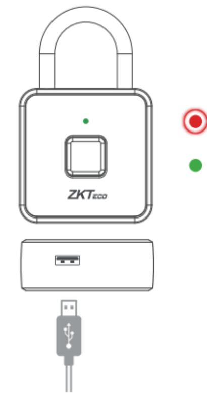
When charging, remove the silicone USB plug, insert the USB cable and link to any PC/tablet or charge pal. **Red LED** is blinking while charging. After about 60 minutes of charging, **green LED** will light, which means the charging is completed.
