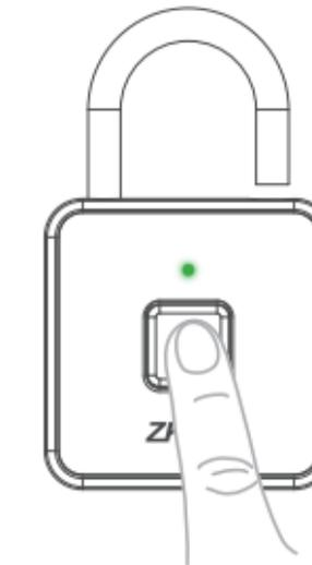
Before adding new fingerprints, use one of the administrator fingerprints to unlock the lock. Under the unlocked state, keep pressing about three seconds until **green LED** blinks.
