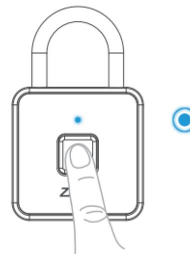
Touch the fingerprint sensor to start, then **blue LED** will blink, which means the lock enters the registration mode.
