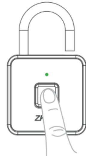
Press with one registered finger on the sensor, **green LED** will light if the verification is correct, then the lock will unlock automatically. If **red LED** lights, please try again more carefully.
