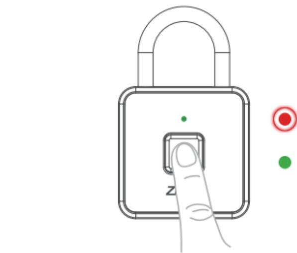
Then loosen the shackle, keep pressing with the administrator fingerprint on the sensor until the blinking **red LED** turns to **green LED**, which means all fingerprints except the first two (administrator) fingerprints are deleted. Repeat the above delete operation again, all the fingerprints will be deleted.
