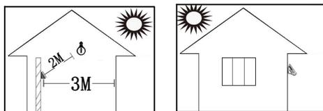
The device can be installed in indoor and outdoor places; the illuminance of external light source is 0-8000LUX. Direct sunlight shall be avoided if the device is installed in outdoor places. Install the device indoors at least 10 feet (3m) away from windows, and 6.5 feet (2m) away from light fixtures.
