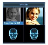
Unfold the blacklist panel of face detection by clicking the **Blacklist** bar and the system will display in the blacklist the blacklist users that it identifies: On the left are face images that it detects and on the right are reference images at registration, as shown in the above figure.
