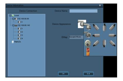
When adding device succeeds, the chosen visual icon for the device will be displayed on the map. You can drag the location of the device icon by moving the mouse cursor to the device icon, pressing and holding the left button of the mouse. Exit editing. After the device is armed, the device icon will blink when there is an alarm input signal. You can double-click the device icon or drag the icon to the video play window to play the video in real time.
