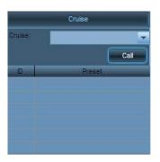
Click **Cruise** bar to display the cruise panel. Select the required camera channel. In the cruise drop-down list, select a cruise. Click **Call**, the Pan-tilt will rotate along the cruise.
