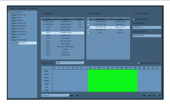
**2.** Check the motion detection area and input alarm settings. For relevant motion detection settings, see <u>5.7 Set Motion Detection</u>. For relevant external alarm inputs, see <u>5.9 Set Alarm Linkage</u>.
