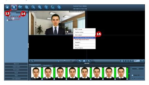
• Note: When facial identification is enabled, click [Play] under Face Event, and the system will automatically compare the current face image captured by IPC with the reference in the system and display a corresponding score. Users on the blacklist will display in the Black List pane as shown in the figure below:
