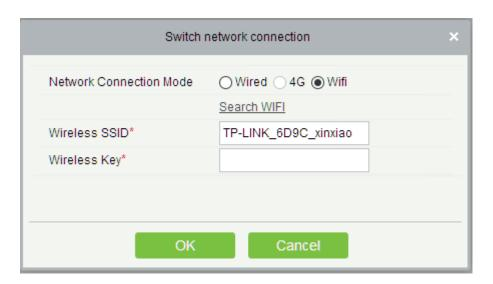
This function is applicable to InBio5 series access control panels, which is used to switch currently network connection mode of control panel.
