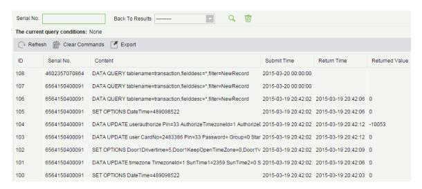
If the returned value is more than or equal to 0, the command is successfully issued. If the returned value is less than 0, the command is failed to be issued.
